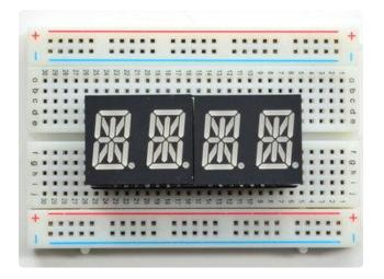
Slot the LED module on top, check again that you have it right way up!
