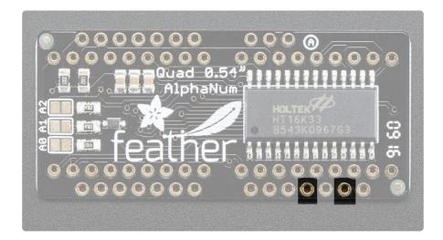
The LED matrix uses only the 3V (second from the right, above) and GND (fourth from the right) pins for power and logic. Current draw depends on how many LEDs are lit but you can approximate it as about 80mA for most uses.
