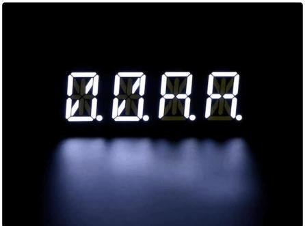
Upload to your Arduino, and open up the Serial console at 9600 baud speed. You'll see each digit light up all the segments, then the display will scroll through the 'font table' showing every character that it knows how to display. Finally, you'll get a notice to start typing into the serial console. Type a message and hit return, you'll see it scroll onto the display!
