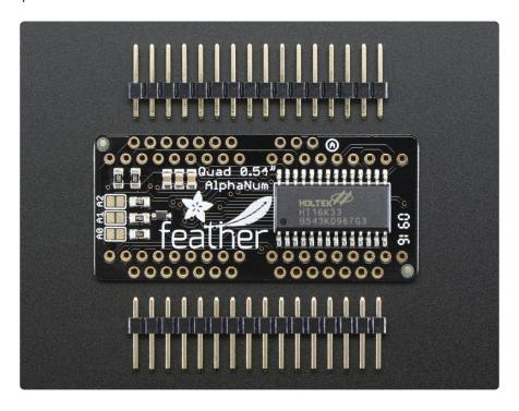
The LEDs themselves do not connect to the Feather. Instead, a matrix driver chip (HT16K33) does the multiplexing for you. The Feather simply sends i2c commands to
