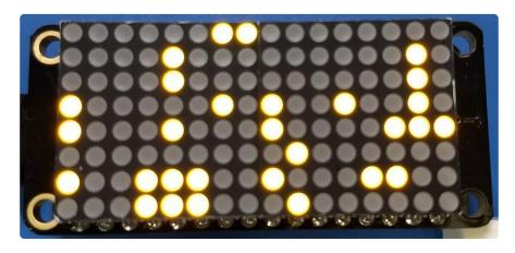
The above command will create the matrix class using the default I2C address of the display (0x70). If you've changed the I2C address (like when using multiple backpacks or displays) you can override it in the initializer using an optional address k eyword argument.
