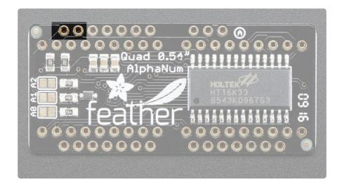
All LED control is done over I2C using the HT16K33 interface library. This means SDA (leftmost) and SCL (to the right of SDA) must be connected, see above for those pins.
