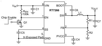
Figure 2. Logic Control with Low Voltage
